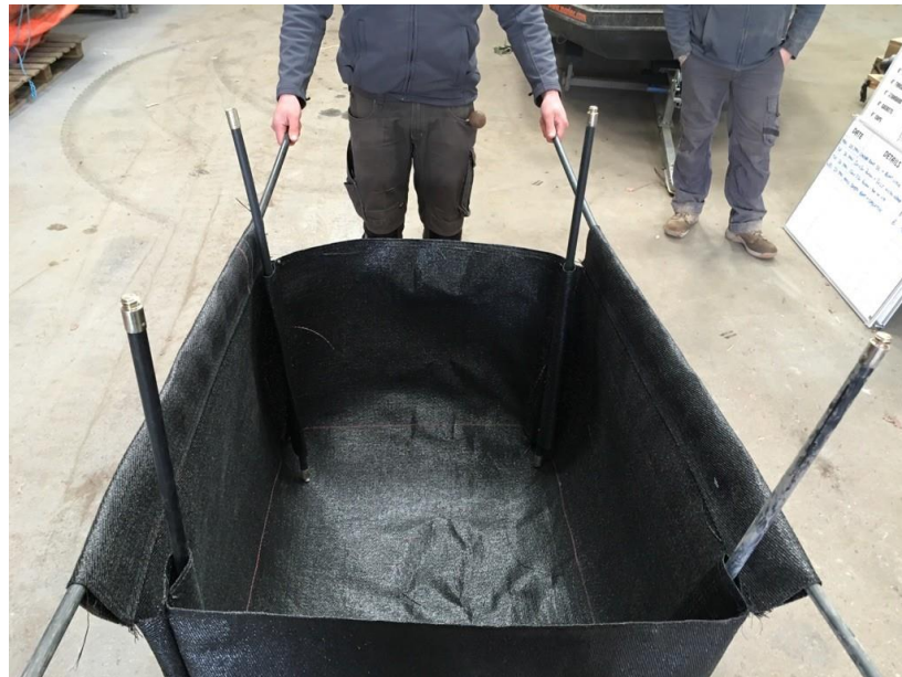
Photograph 2: Prototype Marginal Planting System for City Quay
