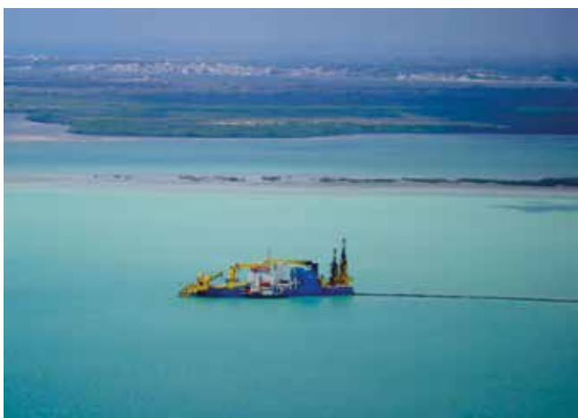
Fig. 3: Dredger operating in proximity to Lamu Old Town for the construction of the first of 32 berths for Lamu Port, with significant turbidity in Manda Bay, April 2019.
