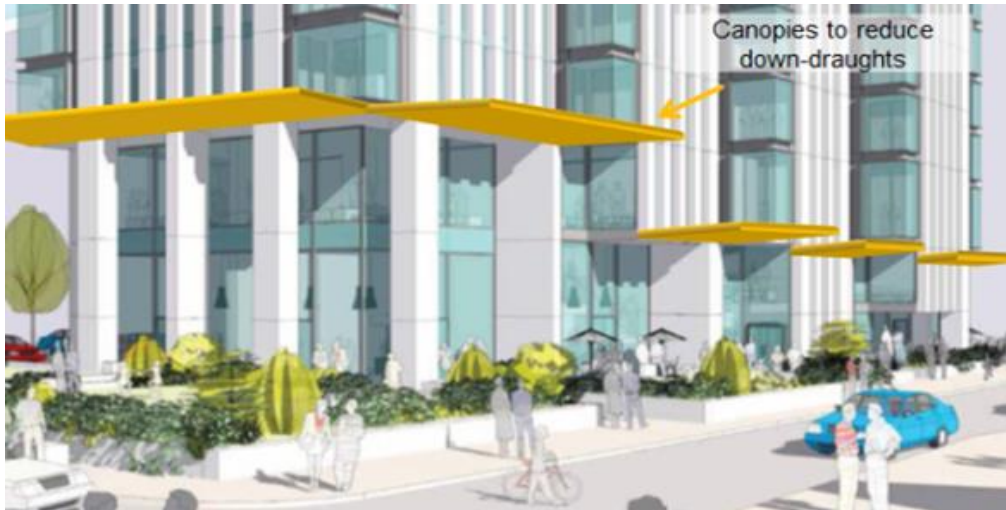
Solid canopies tend to be effective against down drafted winds
