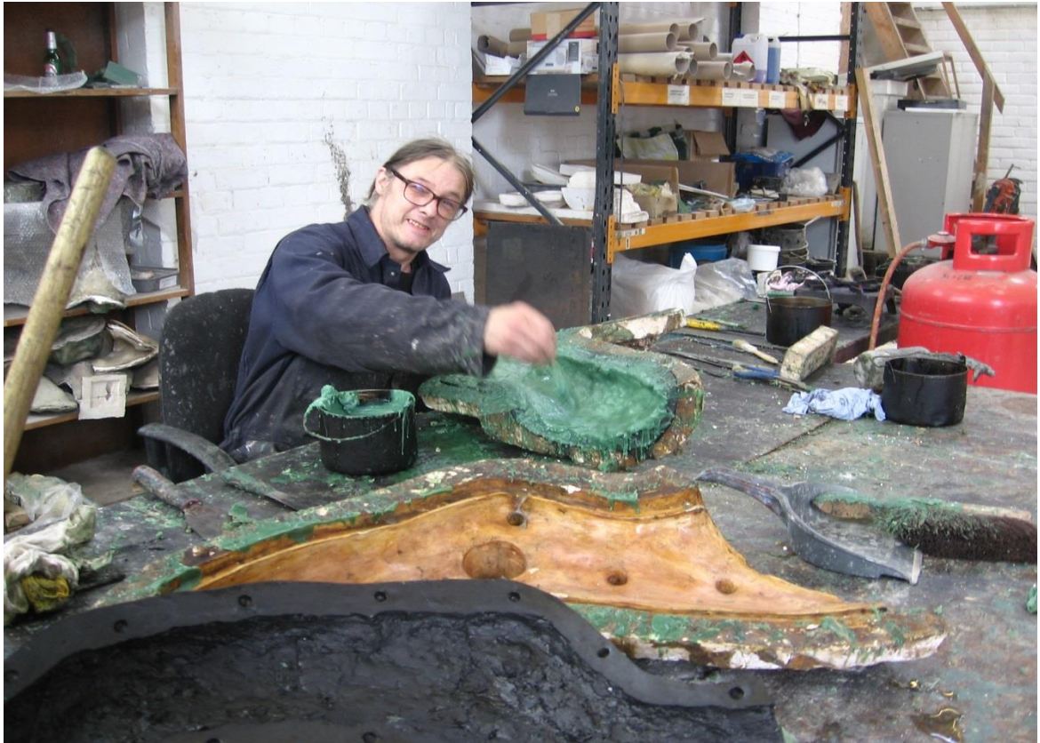
FABRICATING MOULDS FOR CAST BRONZE STATUARY, CASTLE FINE ARTS, BRIDGEWATER STREET
