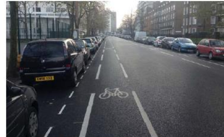
Advisory lanes on two-way streets with no centre-line – wide (left) or buffered (right) to account for parked cars
